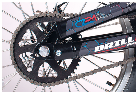
Tensioning of the chain by means of eccentrics on the swinging fork on the rear wheel axle.
