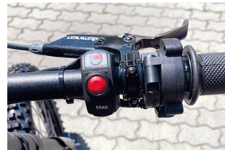
Combined On/Off switch and switch of driving modes (maps).
