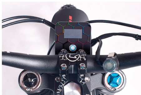
Digital display of battery level, selected map, speed, distance travelled, engine speed and temperature.
